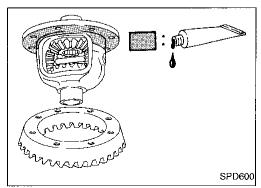
6. Apply locking agent [Locktite (stud lock) or equivalent] to contacting surfaces of ring gear and differential case, then place differential case on ring gear.
