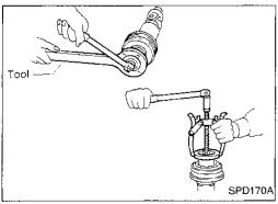
Remove locking nut using Tool.
