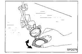
3. Check friction discs or plates for warpage.
