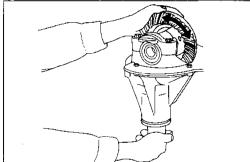
Hold companion flange steady and rotate the ring gear in both directions.
