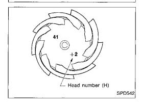
12. Correct the pinion height washer size by referring to the "pinion head number".
