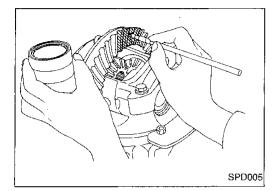
Thoroughly clean ring gear and drive pinion teeth.
