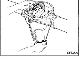
Hold companion flange steady and rotate the ring gear in both directions.
