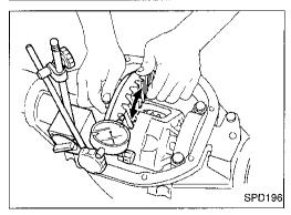
15. Measure ring gear-to-drive pinion backlash with a dial indicator
