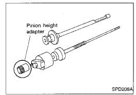
7. Place the J34309-14 pinion height adapter onto the gauge plate and tighten it by hand.
