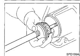
Assemble the front pinion bearing inner cone and the J34309-2 gauge anvil. Assemble them together with the J34309-1 gauge screw in the final drive housing. Make sure that the pinion height gauge plate, J34309-16, will turn a full 360 degrees. Tighten the two sections together by hand.
