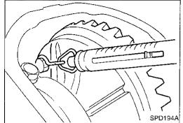
7. Measure the turning torque of the carrier at the ring gear retaining bolts with a spring gauge, J8129.
