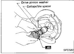
6. Install drive pinion washer, collapsible spacer and drive pinion in gear carrier.
