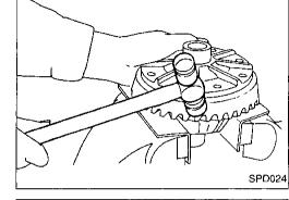
4. Punch off pinion mate shaft lock pin from ring gear side. Lock pin is calked at pin hole mouth on differential case.
