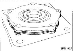
3. Place all of the original side retainer adjusting shims onto the side bearing retainer that goes at the ring gear end of the carrier.
