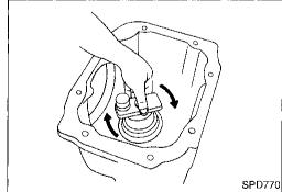
Measure the turning torque at the end of the J34309-2 gauge anvil using Tool.
