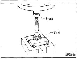
10. Pull out rear bearing inner cone with a press and Tool. Tool number: ST30031000 (J22912-01)
