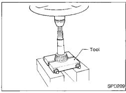
13. Remove pinion rear bearing inner cone and drive pinion adjusting washer.
