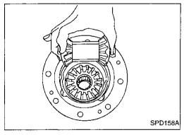
Install pinion mate gears, pinion shaft and thrust block to differential case A.
