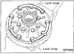
2. Spread out lock straps and loosen ring gear bolts in a criss-cross fashion.
