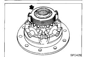
Install side gear to pinion mate gears.
