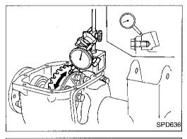
Ring gear runout
