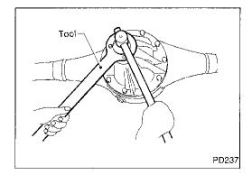
Apply multi-purpose grease to cavity at sealing lips of oil seal. Press front oil seal into carrier. Tool number:
