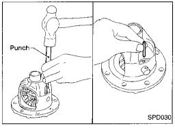
4. Install pinion mate shaft lock pin with a punch.
