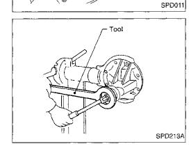
Remove drive pinion nut with Tool.
