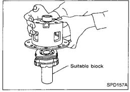
Install differential case A over side gear, discs and plates assembly.
