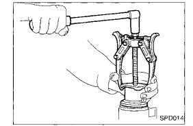
Remove pinion nut with Tool. Tool number: ST38060002 (J34311)
