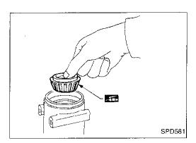
4. Place pinion front bearing inner cone in gear carrier.
