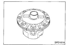
12. Tighten differential case couple screws.
