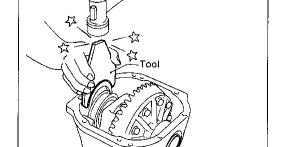
Use Tool to place original carrier side bearing preload shims on the carrier end, opposite the ring gear.
