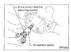
Place drive pinion bearing spacer, drive pinion bearing adjusting washer and drive pinion in gear carrier.
