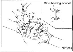
13. Drive in side bearing spacer with Tool.
