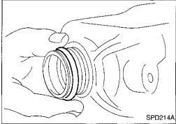
Reinstall all of the original side bearing adjusting shims on the carrier side, away from the ring gear.
