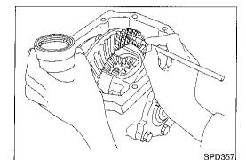
Thoroughly clean ring gear and drive pinion teeth.
