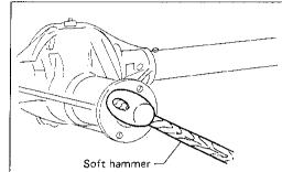
Insert companion flange into drive pinion by tapping the companion flange with a soft hammer.
