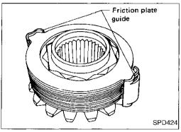
4. Install friction plate guides.
