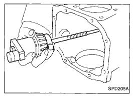
Remove the J34309 pinion preload shim selector tool from the final drive housing and disassemble to retrieve the pinion bearings.
