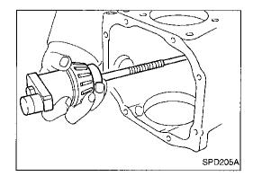
13. Remove the J34309 pinion preload shim selector Tool from the final drive housing. Then disassemble to retrieve the pinion bearings.
