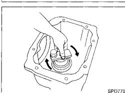
Turn the assembly several times to seat the bearings.
