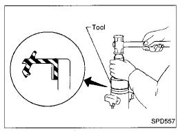
Apply multi-purpose grease to cavity at sealing lips of oil seal. Install front oil seal.
