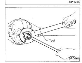
Tighten pinion nut to 127 N·m (13 kg-m, 94 ft-lb).
