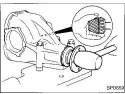
7. Insert companion flange into drive pinion by tapping the companion flange with a soft hammer.
