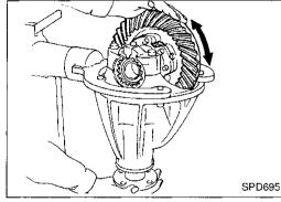
Usually the pattern will be correct if you have calculated the shims correctly and the backlash is correct. However, in rare cases you may have to use trial-and-error processes until you get a good tooth contact pattern. The tooth pattern is the best indication of how well a differential has been set up.
