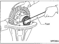
4. Remove side bearing adjuster with Tool. Tool number: ST32580000 (J34312)
