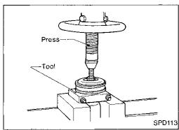
5. Remove center bearing using Tool and press.
