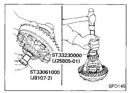
Reinstall the carrier side bearing using Tools J25805-01 and J8107-2. Press on the bearings.
