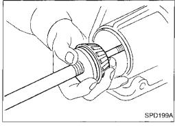
4. Install the J34309-2 gauge anvil with the front pinion bearing into the final drive housing and assemble it to the J34309-1 gauge screw. Make sure that the J34309-16 gauge plate will turn a full 360 degrees, and tighten the two sections by hand.
