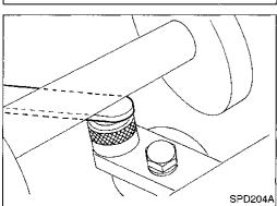
10. Select the correct standard pinion height adjusting washer thickness using a standard gauge of 2.5, 3.0, or 3.5 mm (0.098, 0.118, or 0.138 in) and J34309-101 feeler gauge. Measure the distance between the J34309-12 "H233B" pinion height adapter and the arbor.
