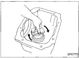
5. Turn the assembly several times to seat the bearings.
