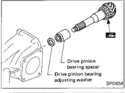
6. Place drive pinion bearing spacer, pinion bearing adjusting washer and drive pinion in final drive housing.
